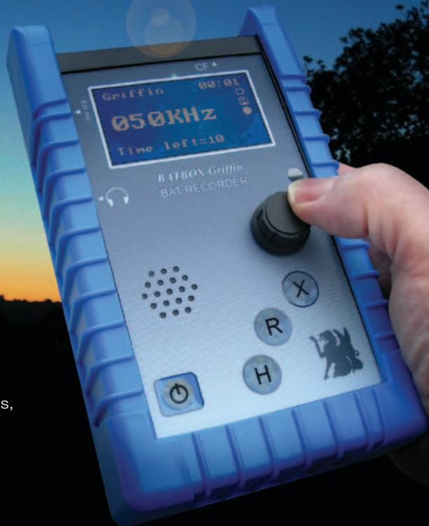
The **Griffin** has been designed to provide all the required functions for studying and surveying bat populations, whilst being easy to use in the dark and without the necessity for the usual connecting leads to recording equipment. Recording time is limited only by the capacity of the Compact Flash card used. The advanced design gives the user setup options, and many automatic features allow use by non-specialist operators.
